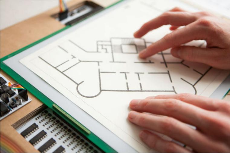
**Fig. 1.5** The third prototype of the *Audio-Tactile Map* featured multi-touch and multi-hand tracking based on open-sourced projected capacitance touch technology. A tactile map was placed on the sensor panel. Audio recordings were triggered when the users double tapped locations with their fingertips
